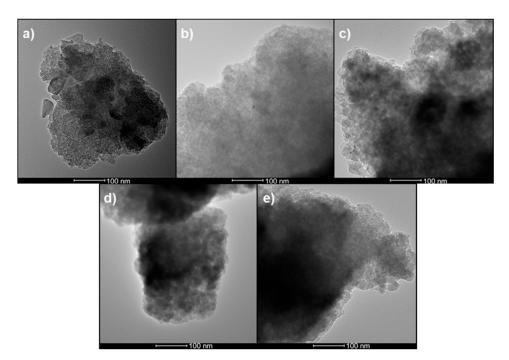
**Figure 1.** High resolution transmission electron microscopy (HRTEM) images of non-ordered mesoporous silicate glasses (MSGs): (a) Undoped-MSG; (b) 5 wt% Ag-MSG; (c) 5 wt% Cu-MSG; (d) 5 wt% Zn-MSG; (e) 5 wt% Ce-MSG. Scale bar = 100 nm.
