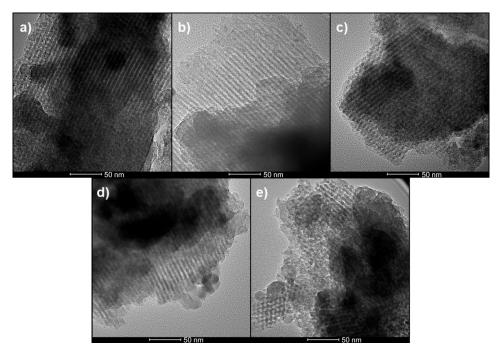
**Figure 2.** HRTEM images of ordered MSGs: (**a**) Undoped-MSG; (**b**) 5 wt% Ag-MSG; (**c**) 5 wt% Cu-MSG; (**d**) 5 wt% Zn-MSG; (**e**) 5 wt% Ce-MSG. Scale bar = 50 nm.
