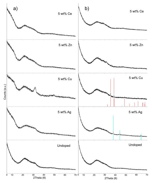
**Figure 6.** X-ray diffraction (XRD) spectra of: (**a**) Undoped and doped non-ordered mesoporous glasses; (**b**) undoped and doped ordered mesoporous glasses.
