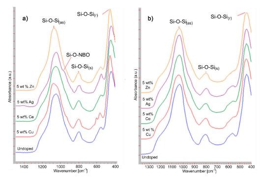
**Figure 5.** Fourier transform infrared spectroscopy (FTIR) spectra of: (**a**) Non-ordered mesoporous glasses; (**b**) ordered mesoporous glasses. (r) Shows rocking, (as) is asymmetric and (s) is symmetric.
