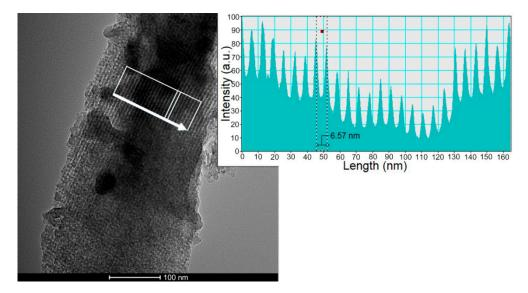
Figure 3. Pore size determination of an ordered MSG.
