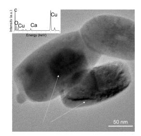
**Figure 7.** Cu included nanoparticles in HRTEM. Inset energy dispersive X-ray (EDX) profile acquired on the particle.
