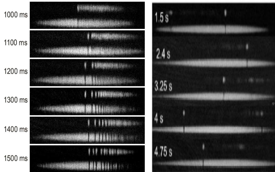
➤ **Hamburg:** Phase-imprinting of a **dark soliton** in state  $|1, 0\rangle$  and **filling** the density dip with atoms in state  $|2, 0\rangle$
