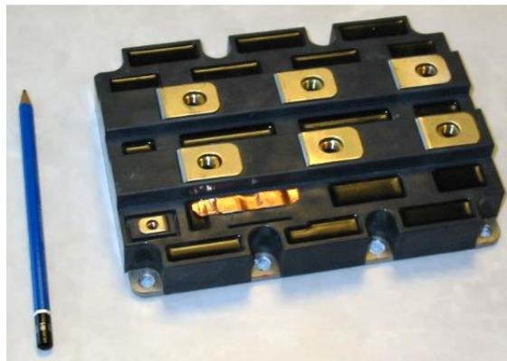
Fig. 1-2. Transistor IGBT [4]
