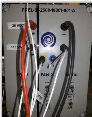
Figura 6-81. Power Supply RARO Box.
