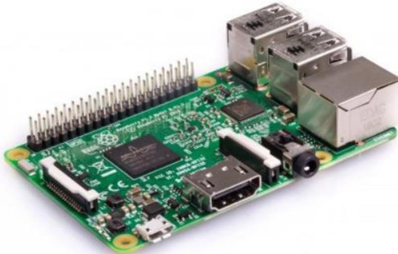
Figura 5. Raspberry Pi3 Model b
