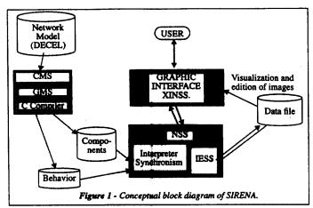
SIRENA allows simulation of general neural networks, and can be considered as functional simulator in which the description and use of general macromodels is possible and simple. However, its development has been focused on the simulation of CNNs.
