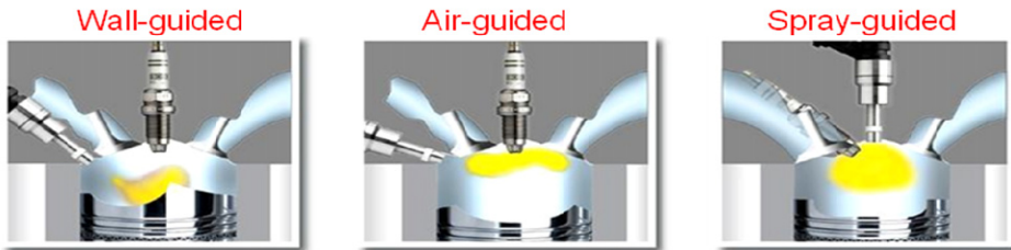
Figure 2: Mixture formation in a GDI engine [29].
