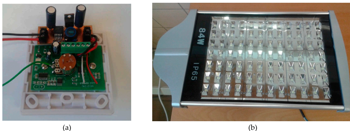
Figure 4. (a) Pulse width modulation (PWM) regulator for the control of the streetlights; (b) Image of a streetlight.
