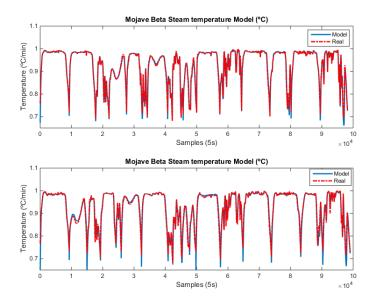
**Figure 14.** Mojave Beta and Alpha: Steam temperature model: (**top**) Mojave Beta model showing real evolution (red dash-dotted) and model output (blue solid); and (**bottom**) Mojave Alpha model showing real evolution (red dash-dotted) and model output (blue solid).
