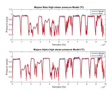
**Figure 15.** Mojave Beta and Alpha: HP Pressure Model: (**top**) Mojave Beta model, showing real evolution (red dash-dotted) and model output (blue solid); and (**bottom**) Mojave Alpha model, showing real evolution (red dash-dotted) and model output (blue solid).
