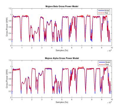
**Figure 16.** Mojave Beta and Alpha: Gross Power Model: (**top**) Mojave Beta model, showing real evolution (red dash-dotted) and model output (blue solid); and (**bottom**) Mojave Alpha model, showing real evolution (red dash-dotted) and model output (blue solid).
