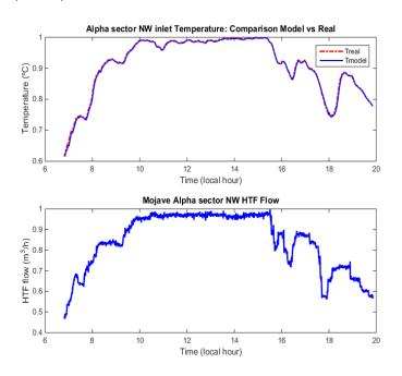
**Figure 13.** Mojave Alpha, inlet temperature of the North-West sector: (**top**) model (solid blue) and real (red dash-dotted); and (**bottom**) HTF flow.
