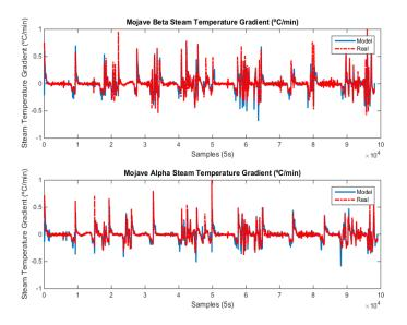
**Figure 18.** Mojave Beta and Alpha: Steam Temperature Gradient: (**top**) Mojave Beta model, showing real evolution (red dash-dotted) and model output (blue solid); and (**bottom**) Mojave Alpha model, showing real evolution (red dash-dotted) and model output (blue solid).
