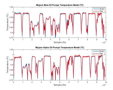
**Figure 17.** Mojave Beta: Oil Pumps Temperature: (**top**) Mojave Beta model, showing real evolution (red dash-dotted) and model output (blue solid); and (**bottom**) Mojave Alpha model, showing real evolution (red dash-dotted) and model output (blue solid).
