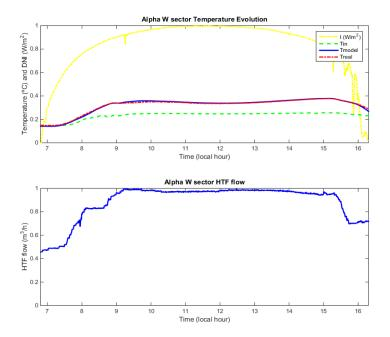
**Figure 8.** Alpha West sector, model vs. real evolution: (**top**) model (blue solid) and real (red dash-dotted); and (**bottom**) HTF flow.
