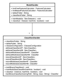
Figure 6: Class diagram of the models handler.
