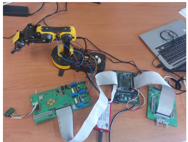
Fig. 3. Complete setup with the yellow robotic arm, AER_Robot board (left) AER_Node board (middle), and monitor board (right).
