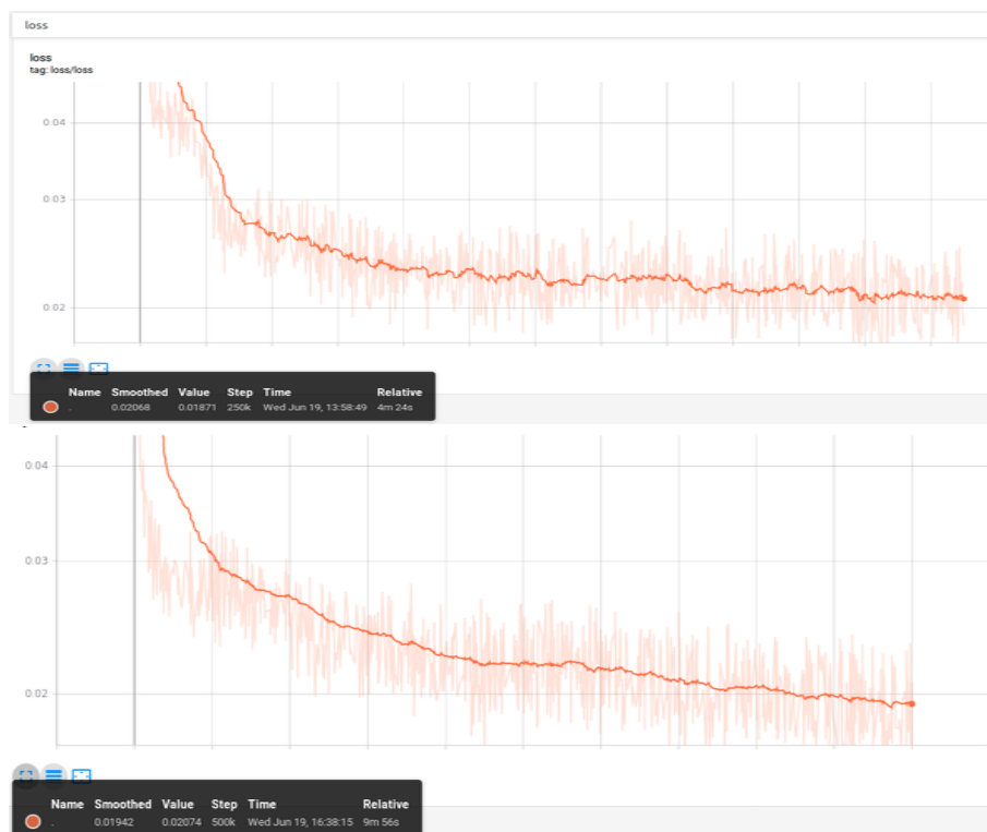
Figure 5.11 Loss functions for different architectures in descendent order inside the lists. LR:0.01, Layers: [10-10,30-30], Steps:[250000,500000], final loss: [0.02068, 0.01942] and test accuracy: [85.2%, 85.6%].
