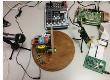
Fig. 1. Completed setup with DC motor, bio-inspired cochlea system (up righth corner), monitor/logger system (down right corner) and DVS128 silicon retina (middle).
