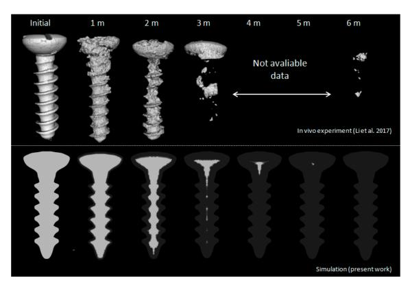
**Figure 4.** Validation of the simulation of magnesium screw degradation obtained by the mathematical modeling presented by Sanz-Herrera et al. [118] (**bottom**), compared with the experimental setup by Li et al. [119] (**top**). Reprinted with permission from [118].
