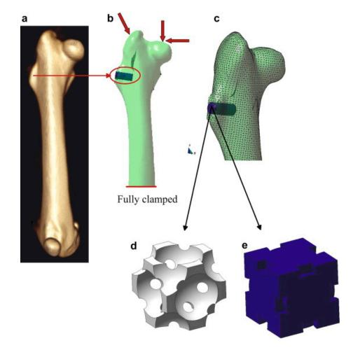
**Figure 2.** Multiscale computer simulation in BTE to predict new bone tissue growth in a unit cell of a predefined scaffold microstructure. (**a**) CT reconstruction of a rabbit femur, (**b**) model of the femur, scaffold implantation, loads and boundary conditions, (**c**) detailed mesh of the model, (**d**) unit cell microstructure of the scaffold solid domain, and (**e**) unit cell microstructure of the scaffold fluid domain. Reprinted with permission from [69].
