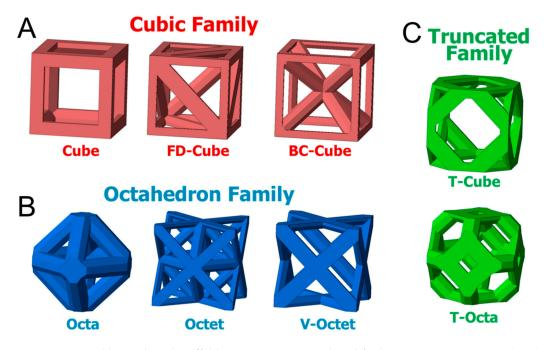
**Figure 1.** Potential lattice-based scaffold microstructures analyzed for bone tissue engineering (BTE) applications. Reprinted with permission from [37].
