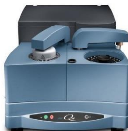
Figure 2.10. DSC Q20 calorimeter
