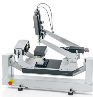
Figure 3.14. Drop Shape Analyser (Krüss)
