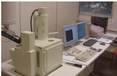
Figure 3.11. JEOL JSM 6460 LV scanning electron microscope
