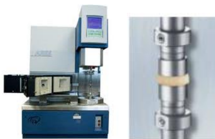
Figure 3.9. RSA-3 rheometer (TA Instruments)
