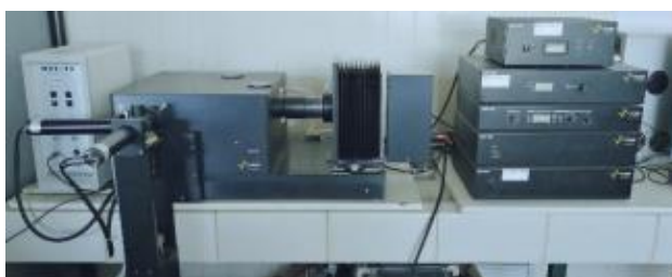
Figure 2.11. Circular dichroism equipment (Biologic Mos-450 spectropolarimeter)
