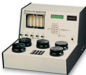
Figure 3.12. Pentapyc 5200e gas pycnometer
