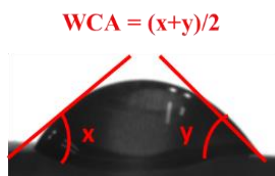
Figure 4.5. Illustration about the calculation of the water contact angle (WCA)
