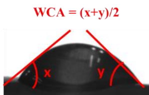
Figure 3.15. Illustration about the calculation of the water contact angle (WCA)
