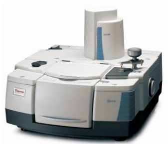
Figure 4.3. iS50 ATR-FTIR spectrophotometer (Nicolet)
