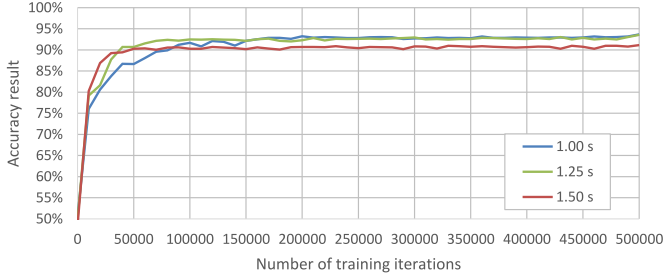
Fig. 9. Accuracy results achieved for each dataset (1s in blue, 1.25 s in green and 1.5 s in red) per 10000 training iterations using the modified version of the LeNet-5 model. Accuracy ratios obtained after 500000 training iterations: 93.68%, 93.57% and 91.14%, respectively, which are better than the ones obtained previously.
