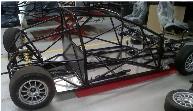
Figura 3-2: Detalle chasis tubular
