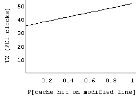
Fig. 12. Evolution of T_2 with probability of cache hit on a modified line.
