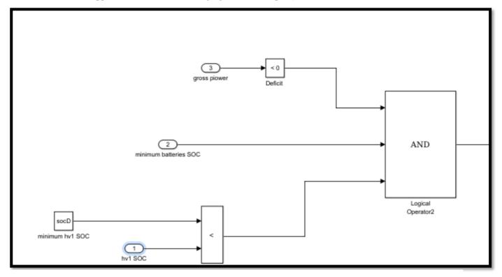
Figure 54. Scheme of discharging HV1
