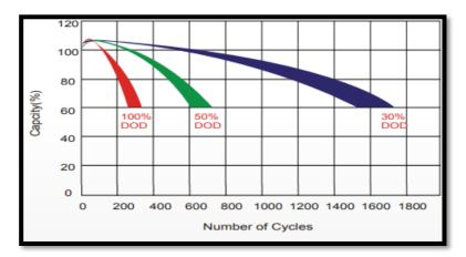
Figure 57. SOC vs Cycle (depending on DoD)
