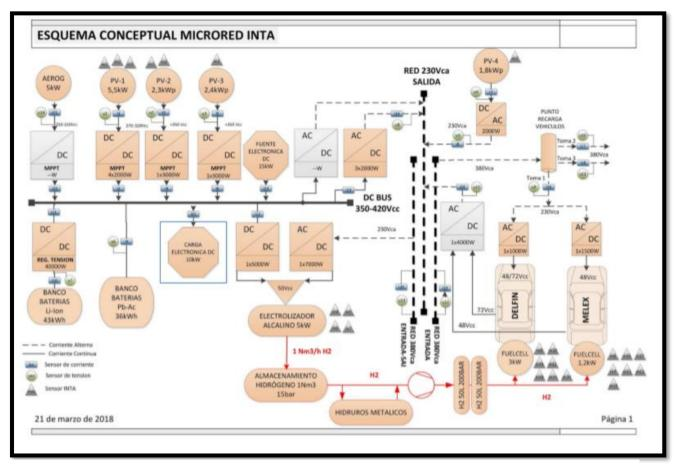
Figure 2. Scheme of INTA microgrid
