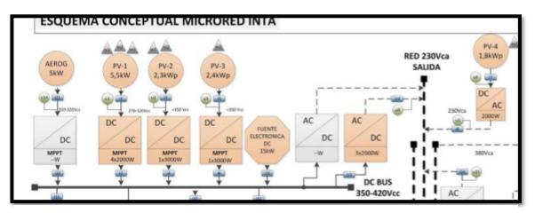
Figure 3. Scheme of mainly inverters
