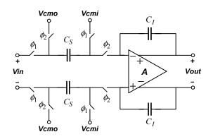
Fig. 4: A switched-capacitor one-sample delaying integrator.
