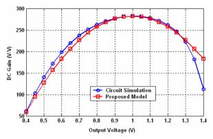
Fig. 1: Amplifier nonlinear dc gain versus its output swing.
