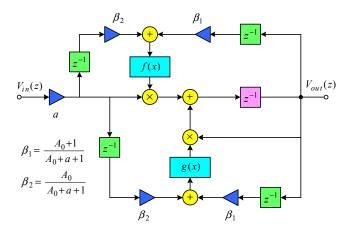
Fig. 5: Modeling the dc gain nonlinearity in a delaying integrator.
