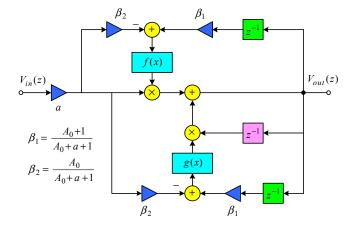
Fig. 6: Modeling the dc gain nonlinearity in a delay free integrator.
