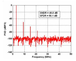
Fig. 7: Output spectrum of a SC gain-stage using the proposed model.
