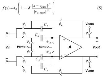
Fig. 2: A switched-capacitor gain-stage.
