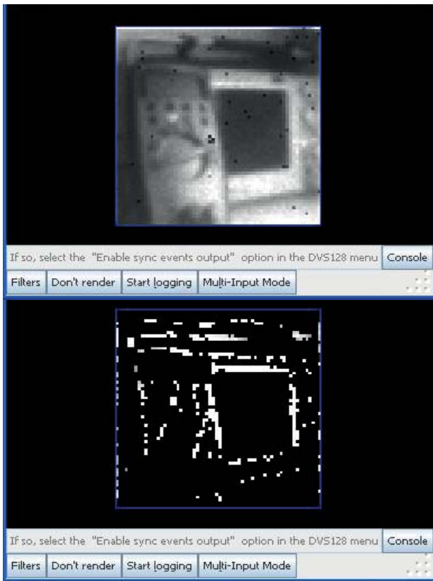
Fig. 12. Custom jAER interface rendering real-time images. We show snapshots of the same scene with the sensor operating in intensity (top) and contrast detection (bottom) modes.
