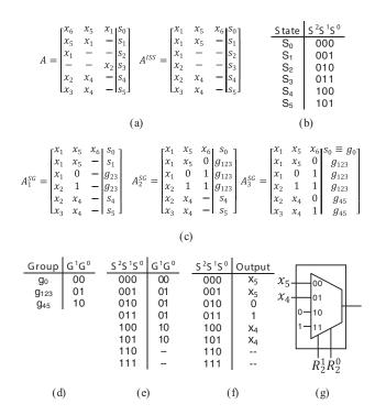
Fig. 2. Example of FSMIM generation. (a) ISS. (b) State encoding. (c) SG. (d) Group encoding. (e) Truth table of the GE of FSMIM-S. (f) Truth table of the second input selector of  $A_3^{\rm SG}$  for FSMIM-S. (g) Second input selector of  $A_3^{\rm SG}$  for FSMIM-T ( $R_2^1$  and  $R_2^0$  are selection bits).
