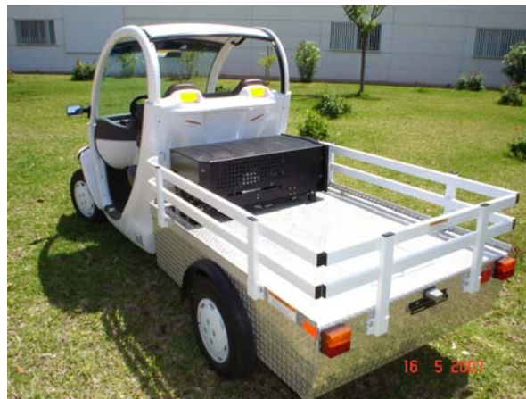
Figure 2. Rear view of the prototype showing the fuel cell.
