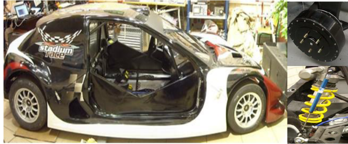
Figure 5 FOX vehicle with custom-made suspension components and in-hub wheel motors (see online version for colours)
