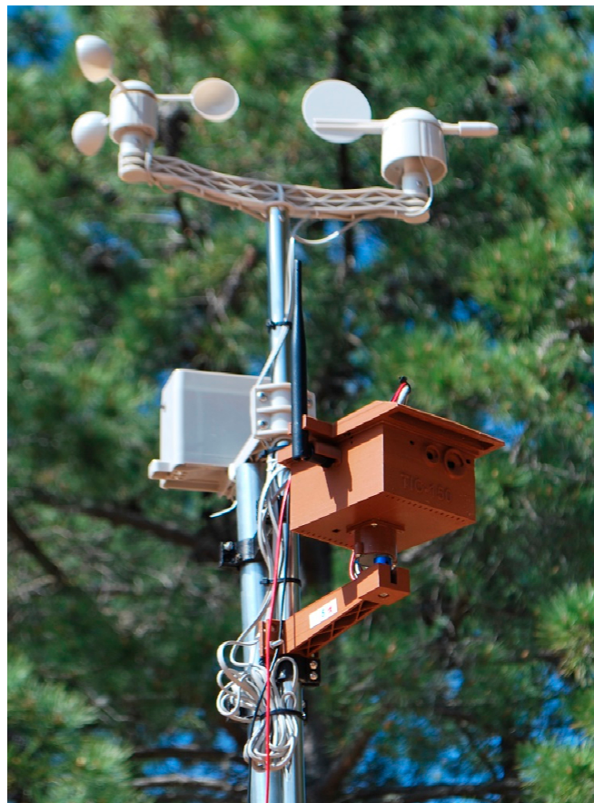
Figure 4. Proposed node fully assembled and deployed in the Doñana National Park.
