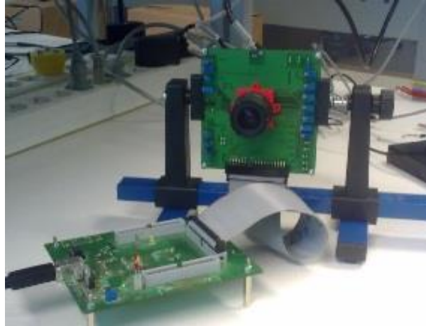
Figure 3 –Experimental setup: vision sensor and data logger.
