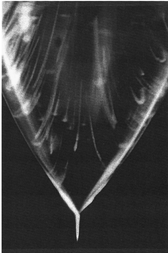
FIG. 4. Conical projections on a meridional plane of particle pathlines in an electrified meniscus of propylenglycol.
