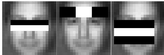
Figure 6: Features composing the first stage of the cascade ‘haarcascade_frontalface_alt.xml’ provided by OpenCV.
