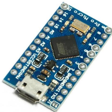
**Figura 7. Arduino Pro Micro.**
