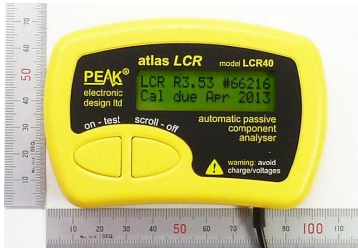
Figura 3-1 Medidor LCR ATLAS LCR40
