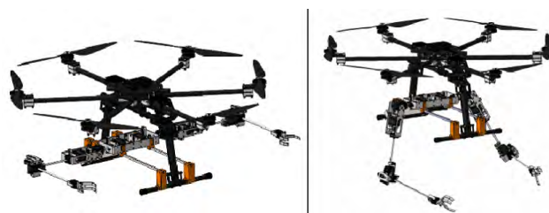
FIGURE 2. 3-D model of the anthropomorphic dual arm integrated in a hexacopter. Take-off/landing (left) and operation (right) configurations.
