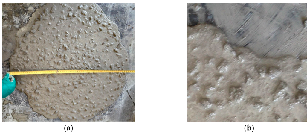
Figure 4. Measured of fresh concrete consistency through flow table tests (a) diameter of flow and (b) border of flow for Mix II.
