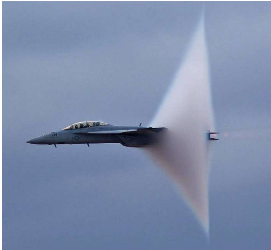
Figure 1.2. Visualized Mach cone due to condensation.
