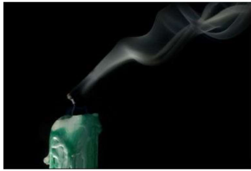
Figure 1.4. In the smoke of a candle it can be appreciated the jump from laminar to turbulent behaviour
