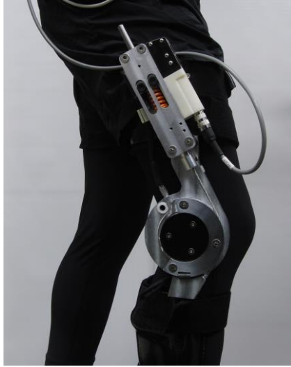
Figure 2-6: Example of an exoskeleton actuator placed in the knee. Yale University [14].
