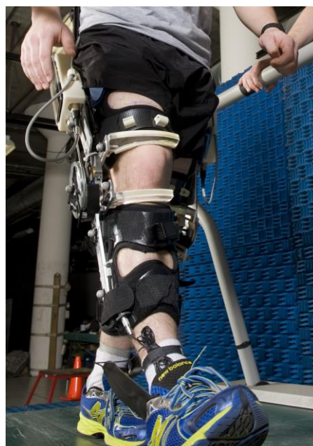
Figure 2-5: Active orthosis for lower limbs. Yale University [14].
