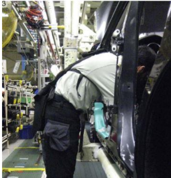
Figure 2-4: Industrial worker wearing PLAD exoskeleton. Graham et al. [10].
