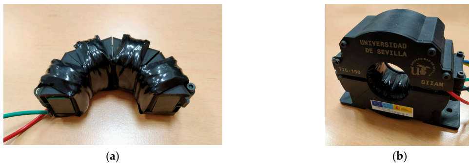
Figure 10. (a) Half ferrite core and its coils; and (b) whole protected coupler.
