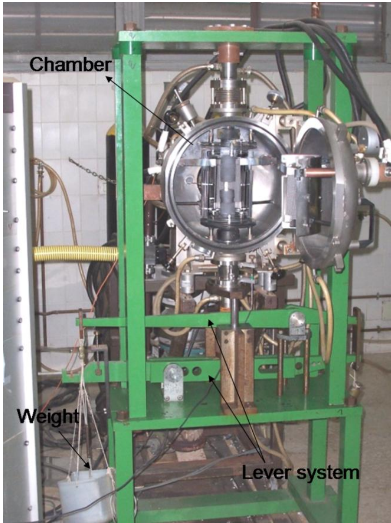
Fig. P5. The prototype creep machine used in this study.
