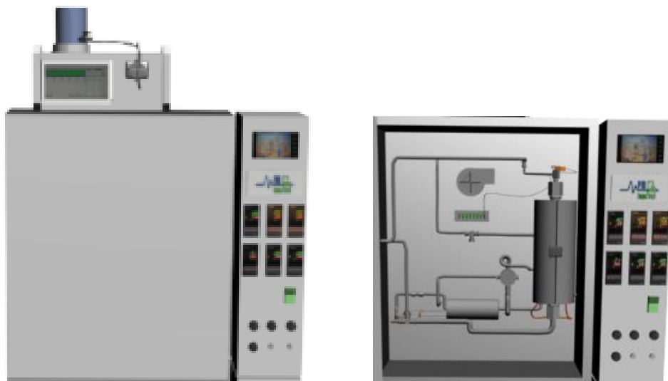
Figure 2.4. Scheme of the reaction system for the evaluation of the catalysts in the WGS reaction
