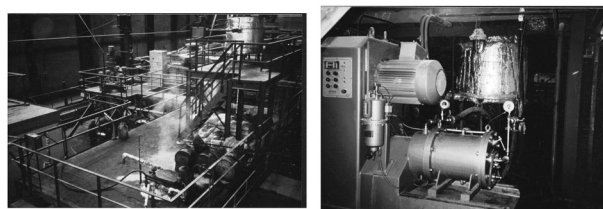
Fig. 53 Pilot plant unit at Rudňany (Slovakia): unit and LME Netzsch attritor in combination with chemical reactor. 821
