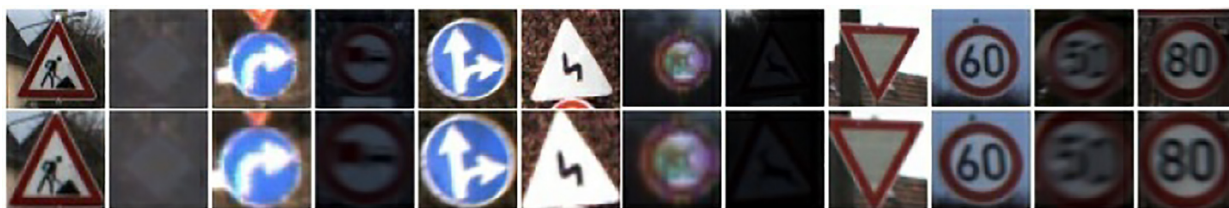
Fig. 5. Spatial transformer network. Input images on the first row and computed output images on the second row.
