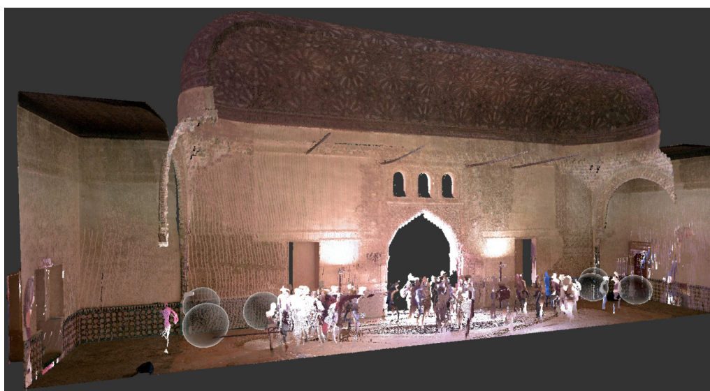
Figure 9. Sala de la Barca: cross section perspective view from the point cloud (gray spheres represent the six scan stations used in the surveying).
