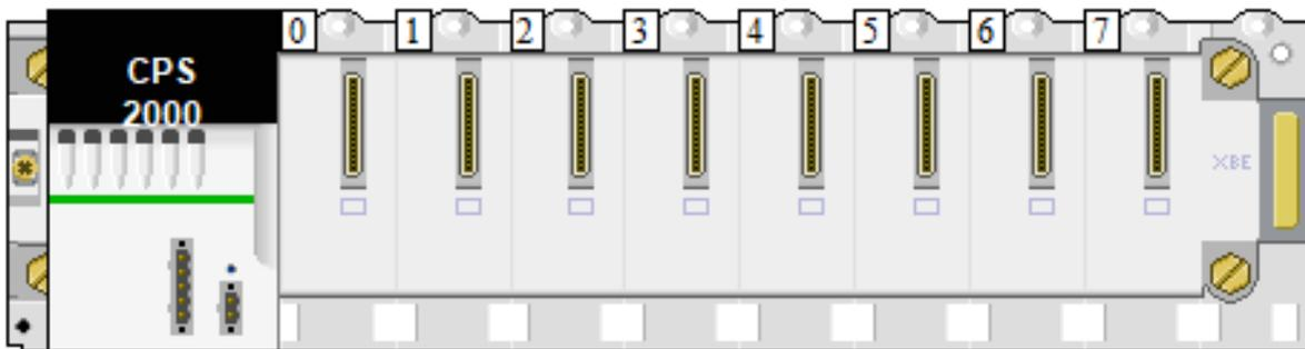
Figura 4-3. Fuente BMX CPS 2000 para PLC Modicon M340 Schneider Electric.
