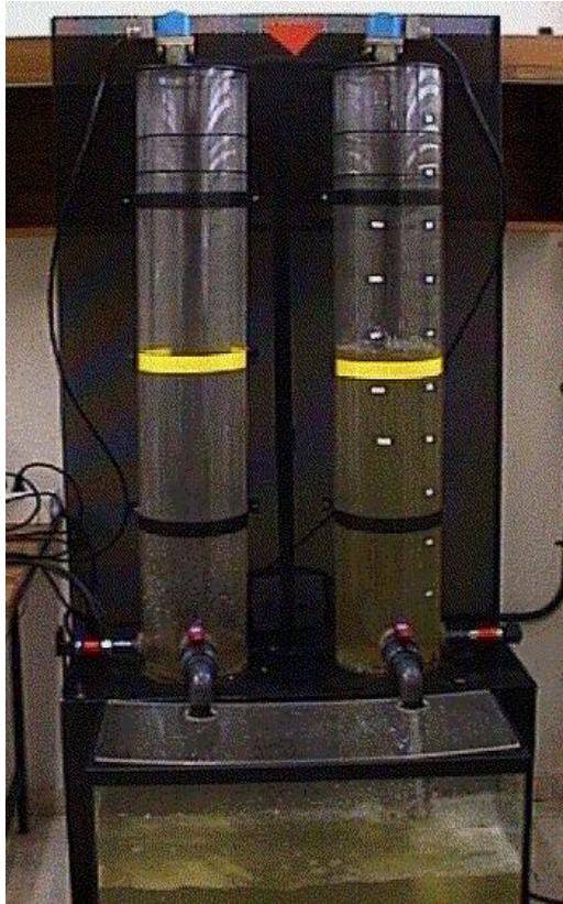
Figure 1. Two-tank level system provided by SUR A&C.
