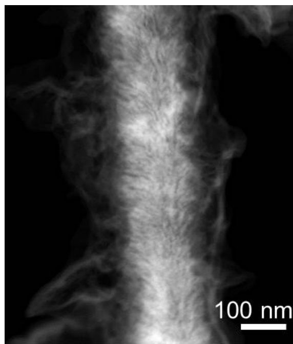
STEM image of a Co thin film supported on polymeric membrane after the catalytic test.
