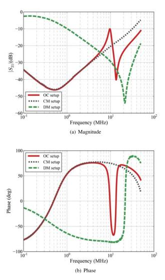
Fig. 4. Magnitude an phase of  $S_{21}$  for the CMC Würth Elecktronik 7446121007 (6.8 mH), listed in Table II and in Table III, when measured using the three configurations of Fig.2.
