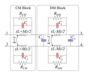
Fig. 5. Equivalent circuit model of a CMC with CM and DM blocks.
