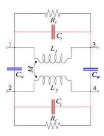
Fig. 1. Circuit model of a common mode choke.
