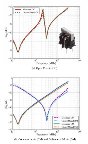
Fig. 9. Measured and approximated  $|S_{21}|$  curves for the CMC shown in the upper figure and listed as KEMET SU9V-R01180 (18 mH) in Table III.
