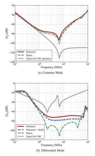
Fig. 12. Measured and approximated  $|S_{21}|$  curves for the EMI filter shown and described in Fig.11.
