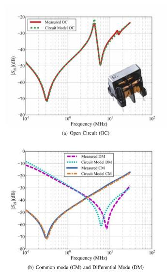
Fig. 10. Measured and approximated  $|S_{21}|$  curves for the CMC shown in the upper figure and listed as MURATA PLA10AN2230R4D2B (22mH) in Table III.
