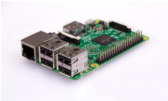
12 Raspberry Pi 3 Modelo B
