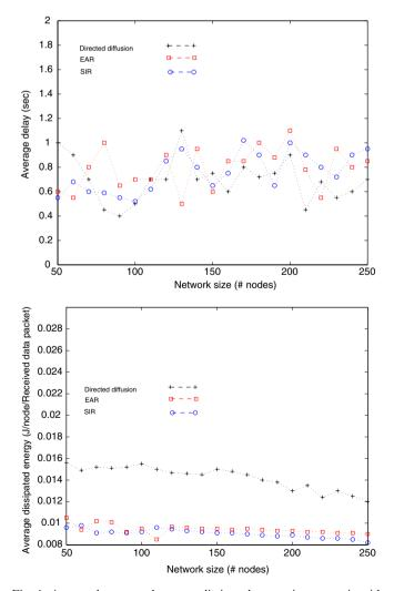
Fig. 4. Average latency and average dissipated energy in a scenario with no simultaneous node failure.
