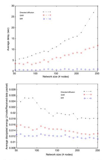
Fig. 5. Average latency and average dissipated energy in a scenario with 20% simultaneous node failures.
