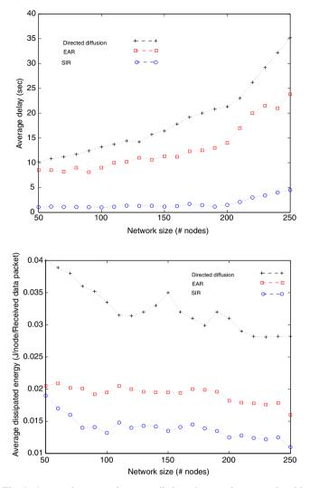
Fig. 6. Average latency and average dissipated energy in a scenario with 40% simultaneous node failures.
