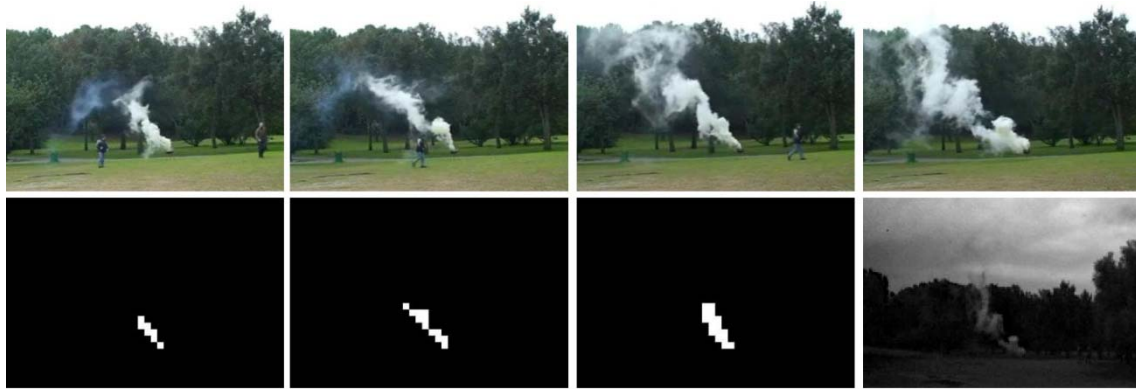
Fig. 13: Smoke segmentation and alarm image from Wi-FLIP .
