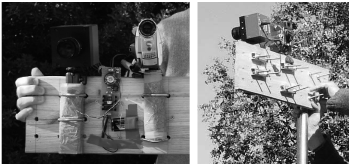
10 Fig. 9: Arrangement of the EyeRIS™ system (on the left in both photos) and the commercial 11 camcorder (on the right in both photos) during the field tests.
