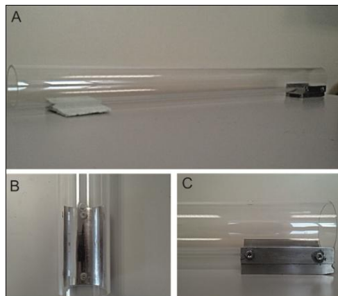
Figure 4.3. Methacrylate CT bed attached to the metallic piece which connects to the CT device
