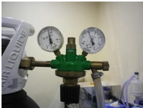
Figure 4.7. Pressure regulator valve. The left barometer shows the pressure of the tank, the right one shows the gas outgoing pressure
