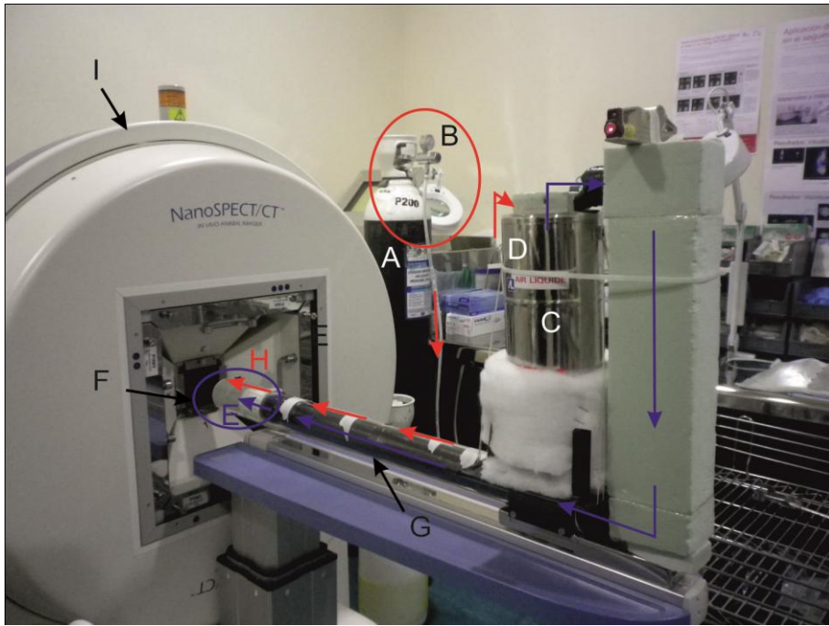
Figure 4.6. Scheme of the cooling system. The red arrows show the nitrogen gas at initial temperature, the blue arrow shows the nitrogen gas pre-cooled with liquid nitrogen
