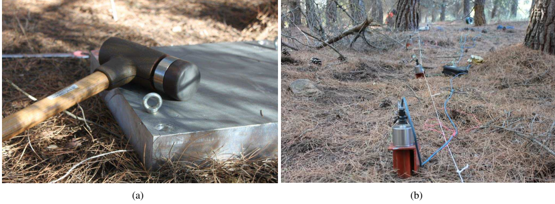
Figure 5: SASW test: (a) impact hammer and aluminium foundation; (b) accelerometers setup.
