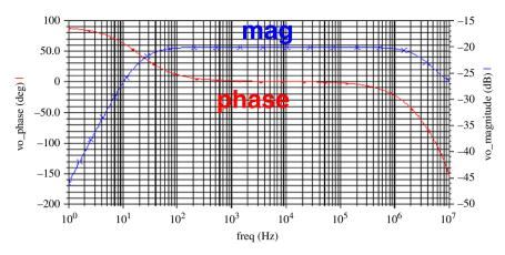
Fig. 4. Instrumentation amplifier magnitude and phase frequency response for 10 mV input amplitude.
