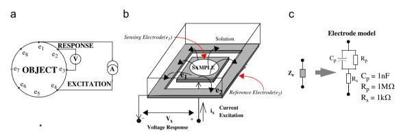
**Fig. 15.** (a) Eight-electrode configuration for Electrical Impedance Tomography (EIT) of an object. (b) Two-electrode system with a sample on top of electrode 1 ( $e_1$ ). The equivalent circuit employed uses  $R_{\text{SAMPLE}} = 100 \, \text{k}\Omega$ .  $Z_x$  includes  $Z_{e1}$ ,  $Z_{e2}$  and  $R_{\text{SAMPLE}}$  resistance. (c) Electrical model for the electrode.
