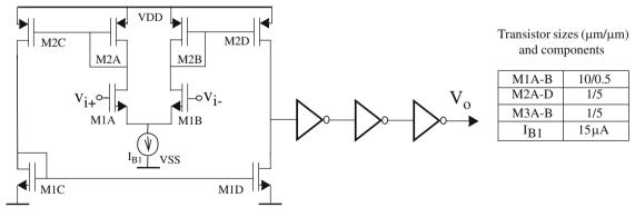
Fig. 10. Comparator circuit schematic.
