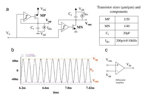
Fig. 5. (a) Full-wave rectifier schematic. (b) Electrical simulations at  $10 \, \text{kHz}$ .  $V_{op}$  and  $V_{om}$  are the upper and lower rectified signals, respectively. (c) Differential-to-single voltage amplifier.
