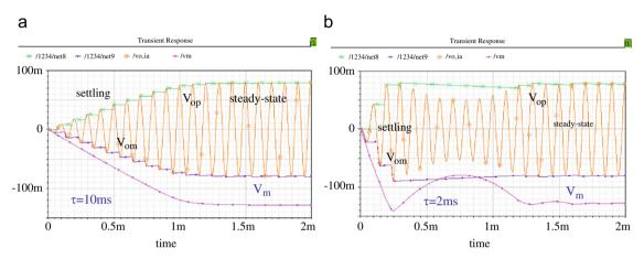
**Fig. 12.** Start-up transient from  $V_m = 0$  to its steady-state, for (a)  $\tau = 10$  ms and (b)  $\tau = 2$  ms, at f = 10 kHz.
