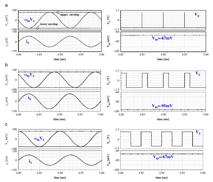
Fig. 13. Waveforms obtained by electrical simulations:  $V_x$  and  $i_x$  are the voltage and current excitation signals.  $V_m$  and  $V_\phi$  are the voltage signals obtained from measurement circuits using (a)  $R_x$ =100 kΩ. (b)  $R_xC_x$ =(100 kΩ|159 pF) and (c)  $C_x$ =159 pF.
