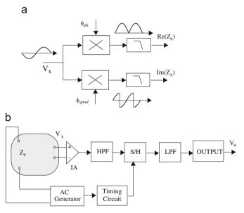
Fig. 1. (a) Coherent demodulation. (b) Synchronous sampling.
