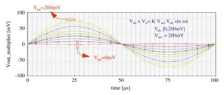
Fig. 8. Simulated multiplier output voltage waveforms.
