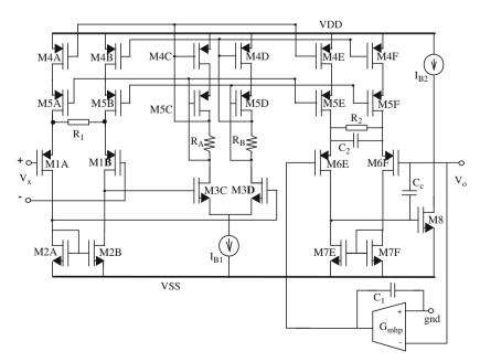
Fig. 3. CMOS instrumentation amplifier schematic.
