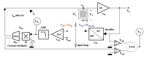
Fig. 11. Open loop system for steady-state stability analysis.
