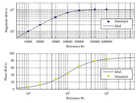
Fig. 14. Magnitude and phase obtained from electrical simulations for  $R_x||C_x$  using  $C_x = 15.9$  pF and  $R_x$  belongs to  $[10 \text{ k}\Omega, 1 \text{ M}\Omega]$  at f = 100 kHz.
